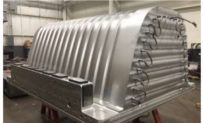
Molds made by Commercial allow the composite materials to be heated and formed
